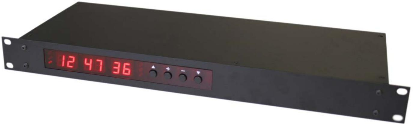
The 5200, 5400 and 5600 series of net time servers provide the time synchronisation solution for complete systems of equipment including computer networks, CCTV security, voice recording, industrial process control, CCC and many other applications requiring accurate time synchronisation.
